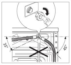
3. Set the hose correctly by loosening the ring nut. After positioning the inlet hose, be sure to tighten the ring nut again to prevent leaks.
